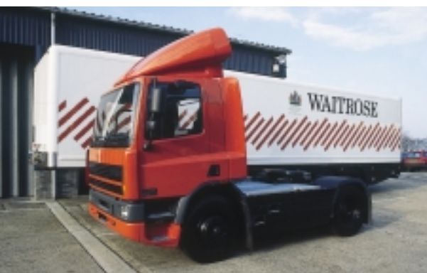
The tractors of our vehicles have aerodynamic additions, while the trailers are low and have rounded corners and side skirts to reduce drag
