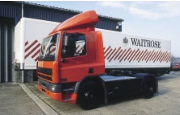
A low silhouette tractor and trailer, with rounded corners and side-skirts to reduce drag
